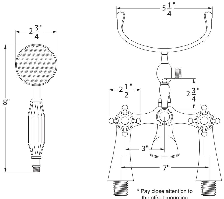
\* Pay close attention to the offset mounting legs. Although the faucet is a 6" spread, the mounting legs install into a 7" spread.
