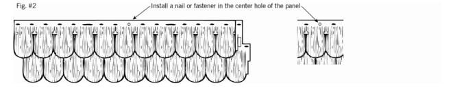
5. If the panel is a partial panel used at either end, a new center hole should be created, by drilling a 1/8" hole in the top flange, near the center of the panel at the same height as the other installation holes (Figure 3).
