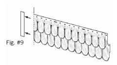
STEP SIX When installing any scallop product into another, hold panel on the left side and the top of the right side. Lower the bottom right corner of the panel about 45 degrees to ease installation (Figure 10).
