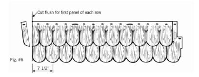
STEP FOUR Working left to right, position and install starter clips on scallops #2, # 5, # 8, and #11. Do not use a clip on the first scallop, as it will interfere with installation. When transitioning from one panel to the other, the first starter clip on the new panel should be positioned 10" apart from the last starter clip on the proceeding panel (Figure 7).
